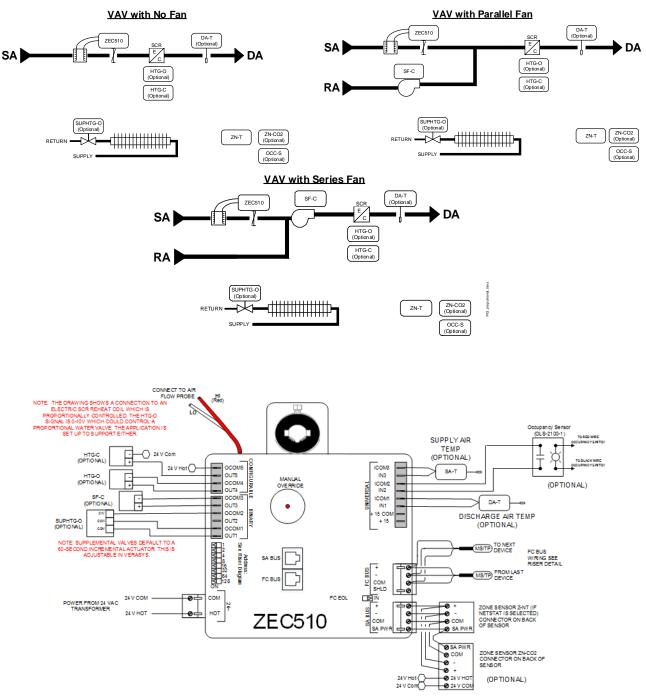
Figure 11: Multizone Unit VAV with Proportional Reheat
