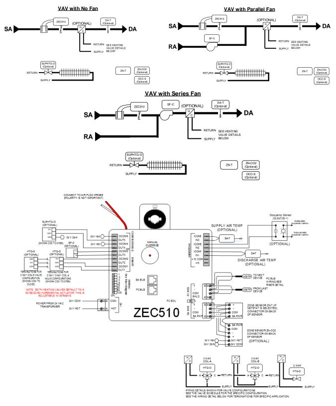
Figure 10: ZEC510 and ZEC500 Controller - VAV with Incremental Reheat Control Wiring Example
